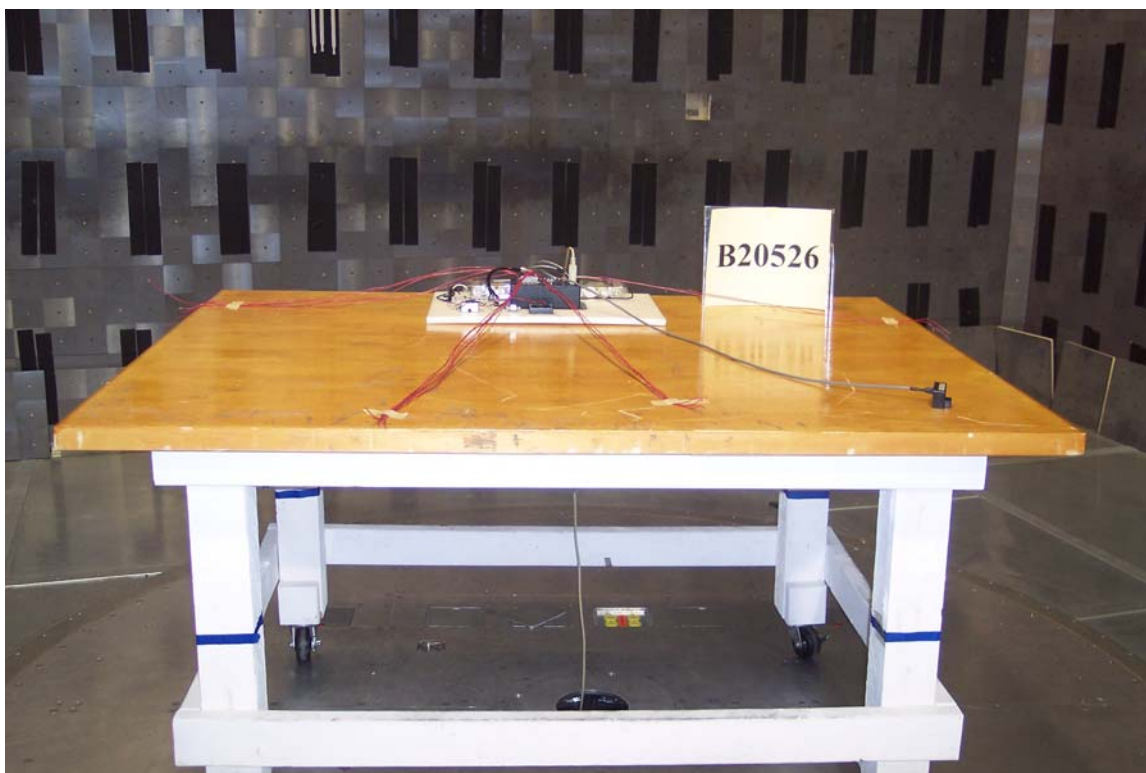
Figure A2: Radiated Emissions Test Setup – Front Side
