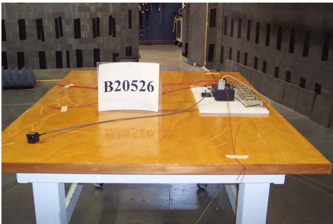
Figure A3: Radiated Emissions Test Setup – Right Side
