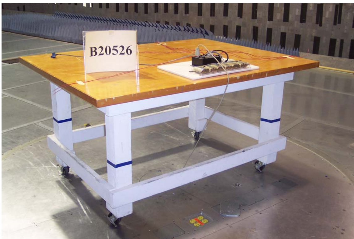
Figure A4: Radiated Emissions Test Setup – Back Side
