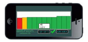
As an accessory to an Elithion BMS, the Wireless Advisor makes the battery status conveniently available to any WiFi enabled device, using any web browser.
